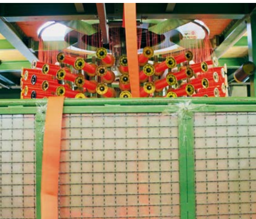
prepared loom for production of orange jacket
