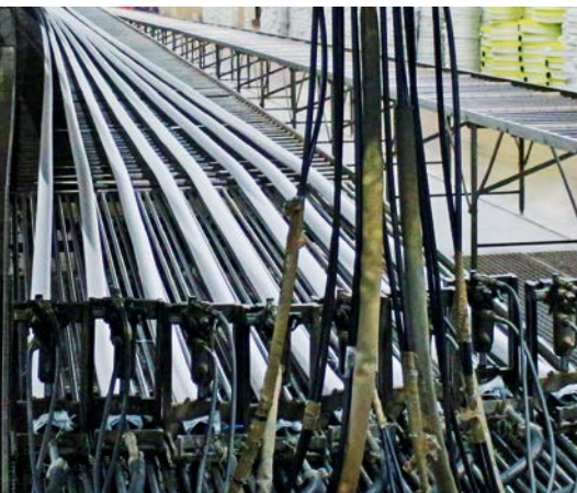
hoses during vulcanizing process
