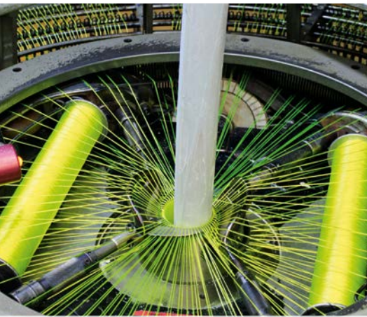
weaving process of jacket with incoming rubberlining
